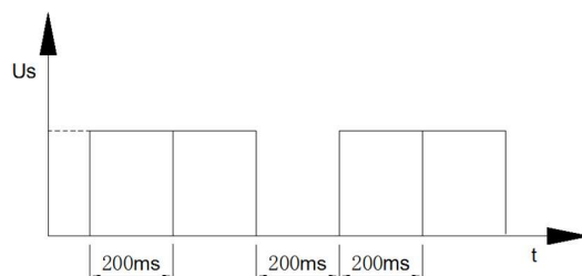
Fig.25 Working principle diagram of shunt tripper
